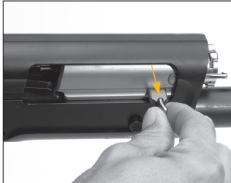
Pull outward to remove the operating handle.
