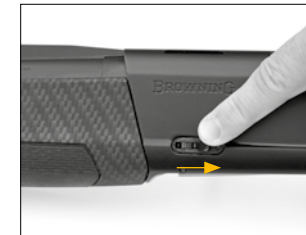
Pull the Magazine Cut-Off rearward to block the magazine.
